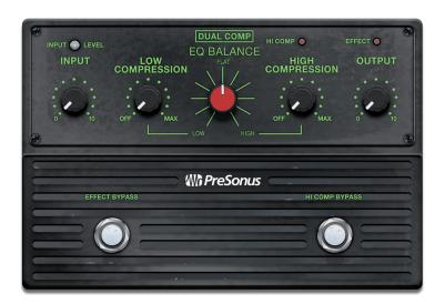
Compress your lows and highs independently for nuanced dynamics processing. Dual Comp's unusual design includes overlapping frequencies and independent controls for the amount of compression. There's no attack control, instead the Dual Comp has fixed fast attack on the high band and a slower attack on the lows. There's even a separate bypass for the highs, so only low frequencies are compressed. It's no wonder its hard-to-find hardware inspiration is coveted by tweaky bassists.
