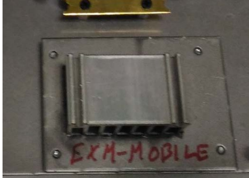
2 Place the 6698 heatsin in the guide.
