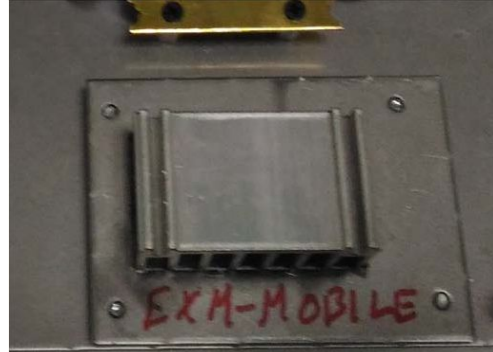
2 Place the 6698 heatsin in the guide.
