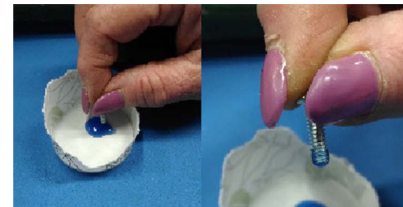
7 Mount 6698 using 2 #8807 screws. Dip the screws in Loctite. Tighten to 4 in lbs.
