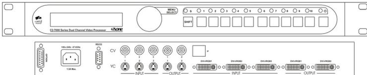
The C2-7100 & C2-7200 feature two independent video processing and scaling engines (CORIO2) and two video mixers for maximum flexibility in handling DVI, RGBHV, RGBS, RGsB, YCbCr, YPbPr, CV and Y/C signals. In addition, the C2-7200 also supports SDI and HD-SDI.
