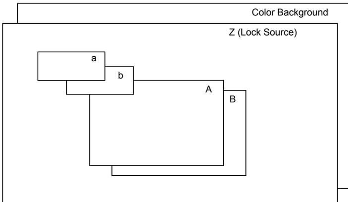
With the exception of the color background layer, the layers can be re-ordered so that different orientations are displayed. For example, the combination shown below could be created which would mean that the Window "A" layer would have primacy over all the others:
