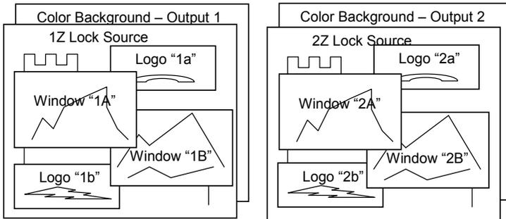
Inputs switched into Windows "A", "B" and "Z" appear on both outputs (in other words, the imagery present in Window 1A is the same as 2A and the imagery present in Window 1B is the same as that present in Window 2B).
