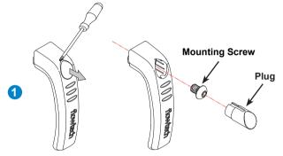
**2.** Using the supplied Hex key, align the mounting screw in the handle with the accessory dock and tighten clockwise, as shown below. Ensure the handle is secure. Insert the plug back into the handle, ensuring the groove is uppermost and it is firmly pushed home.
