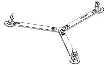
2. Place the tripod foot on the ball of the spreader foot.
