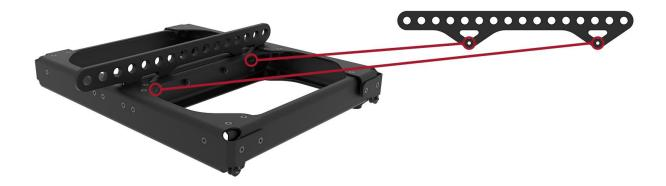
2. Place flybar on top of sub and use M8 X 30 bolts to rig front and rear positions.
