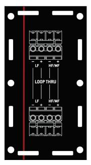
There are two Phoenix connectors on the rear of the KF810. Use one for input, and the other to loop through to other units in the system.
