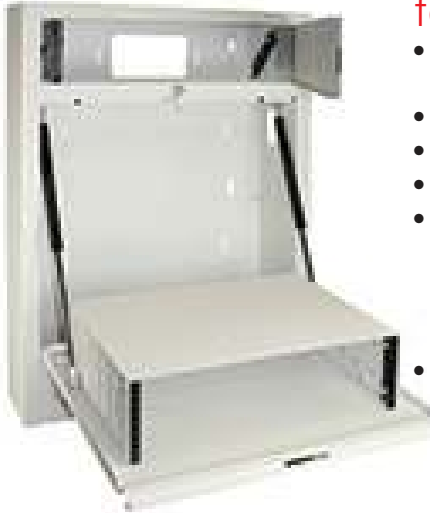
Wall-mount rack with two bays—a hinged pocket door on the upper bay swings open, the lower bay tilts down when opening to the service position (oil-filled dampers control the rate of descent).
