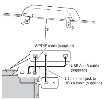
1. Attach the supplied camera with the supplied knurled screws (M3) (x2).
