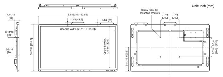
When mounting the monitor, be sure to use a wall-mount bracket that complies with the VESA-compatible mounting method. SHARP recommends using M6 screws and tighten the screws.
