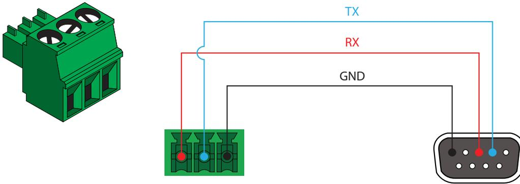
RS-232 is often connected through a DB 9-pin to captive screw connector. The pins will have functions associated with them, some will be unassigned.
