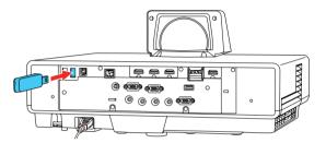
**Note:** The light on the wireless LAN module turns on when the module is installed and operating. The light flashes when the module is communicating over the network.
