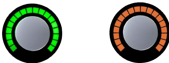
Apollo Solo USB's top panel preamp knob during normal operation (left) and when a Unison plug-in is in the Unison insert of Apollo Solo USB's selected channel (right)
