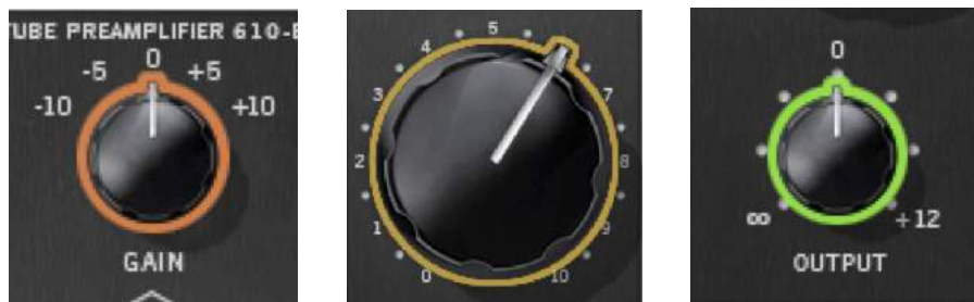
The matching color dot on the parameter in the Unison plug-in interface indicates which gain stage is being controlled by Apollo Solo USB's top panel knob
