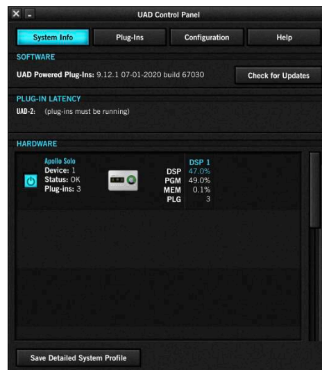
UAD Control Panel with System Info panel selected
