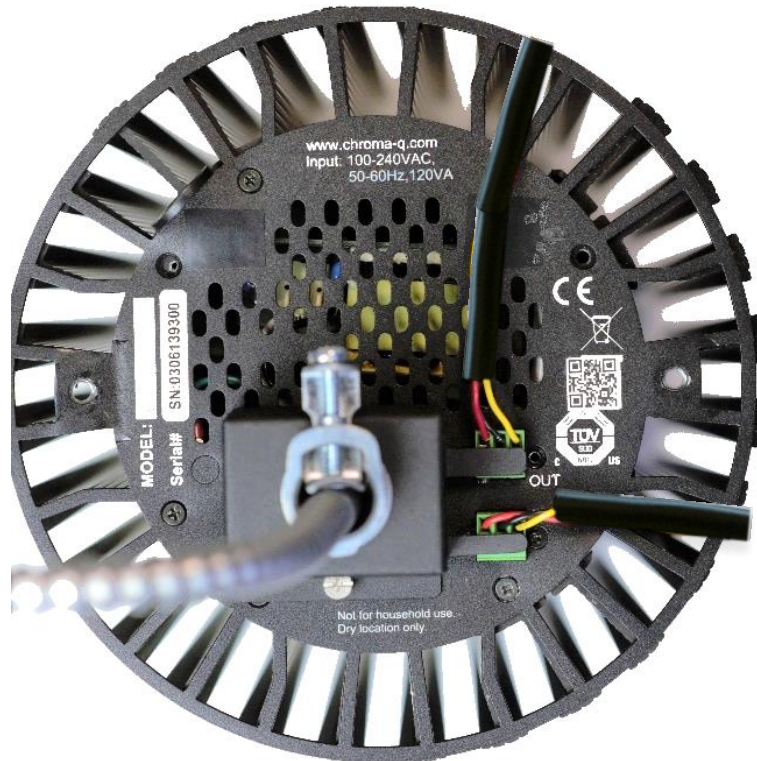
Figure 6: Back Plate of Inspire Terminal Strip after connection
