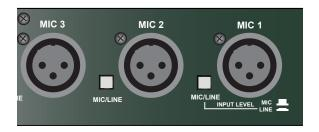
The XLR input for MIC 1,2 and 3 can be configured to be Microphone level or line level. Follow the silk screening on the unit for proper use of the mic/line switch.
