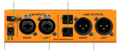
**POWER INPUT -** Connection for the included 15V 400mA power supply.
