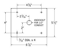
4. After the DTS4T enclosure has been securely mounted, verify that it cannot be dislodged from the mounting surface.
