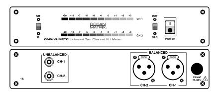
The VUM-2TC is a precision audio level measurement tool for confirmation and/or calibration of line level audio signals. The VUM2TC is factory calibrated and requires no user adjustments. The OMX-VUM2TC is designed to work with either Balanced Audio or Unbalanced audio. Separate connector inputs are provided for either format. Female XLR connectors are provided for the Balanced signals and RCA phono type are provided for Unbalanced audio.
