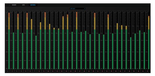
The Meters tab provides up to 32 individual volume meters for each row from the 'Routing' tab, selectable from the drop-down menu.
