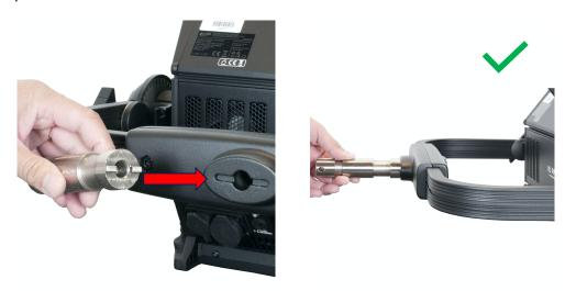
2. Locate the notched face of the junior pin, and hold it against the clamp mounting point located on the top side of the yoke. The notched surface of the junior pin must sit flush against the matching groove on the surface of the clamp mounting point.
