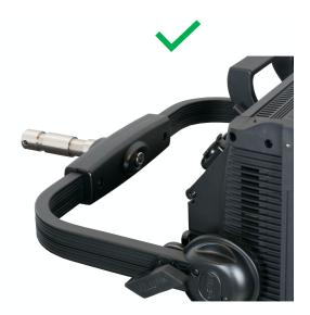
3. Thread the junior pin bolt in through the under side of the mounting yoke, making sure that the bolt engages the threaded hole in the junior pin. Tighten securely with a 10mm hex key. The junior pin is now ready for attachment to a clamp or stand.
