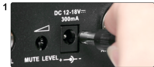
1 Insert the 5.5mm plug into the DC input jack, plug the wall wart into a 120VAC outlet.
