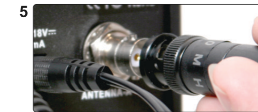
5 Attach the antennas to the antenna jacks
