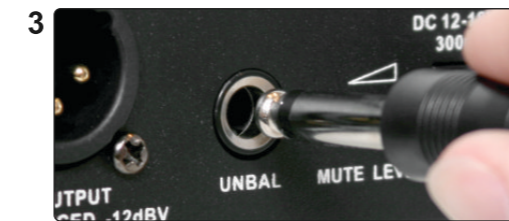
3 Combined Outputs-1/4": Connect one end of a shielded 1/4"M to 1/4"M cable, to the 1/4" Mix output, connect the other end into your system input.
