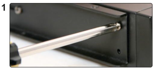
1 Screw one short rack ear on the left side of the first receiver, and one coupler half onto the right side of the same receiver using the provided screws.
