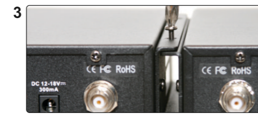
3 Align both receivers so that the coupler halves fit, and screw them together.
