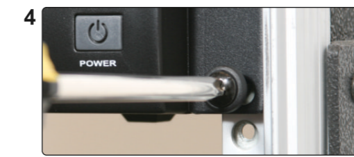
4 Align the dual receivers to the rack and screw into the rack.
