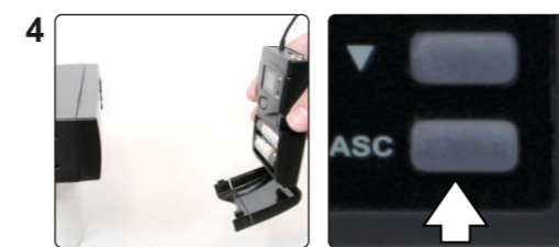
4 With the transmitter turned on, place the transmitter with its IR window (figure 4a) facing the receiver IR window (figure 4b), about 6" away. Press the ADS button on channel 1. This will sync the Transmitter to the Receiver.
