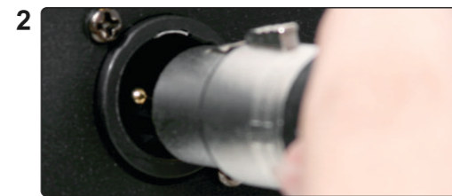
2 Individual Output: Connect a shielded microphone cable to the channel's XLRM output, connect the other end into your mixer input.
