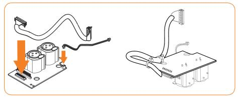
► Attach the digital input board to the loudspeaker electronics, as shown below. The two XLR sockets will only fit into the holes in one orientation.
