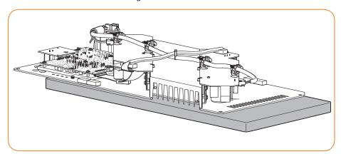
► Carefully remove the sticker from the DIM 1 area of the backplate. Do not remove the other smaller sticker.
