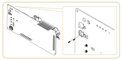
► Carefully pull the analog input board off the loudspeaker electronics, as shown below.
