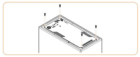
Bring the loudspeaker into an upright position and refit the woofer ring by aligning the pegs with the holes and gently pushing until the woofer ring is fully inserted.
