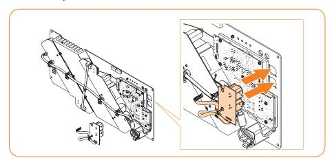
► Fasten the digital input board using the four supplied Torx 8 screws and lock washers on each of the two XLR sockets (ANALOG INPUT and AES3 INPUT) with a torque of 0.5 Nm, as shown below.
