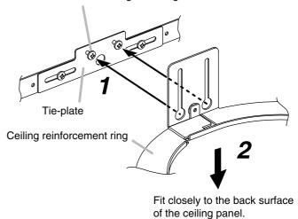
If the ceiling reinforcement ring does not line up accurately with the ceiling mounting hole, adjust its position by either loosening the tieplate mounting screws and sliding the tieplate into correct position, or by shifting the
