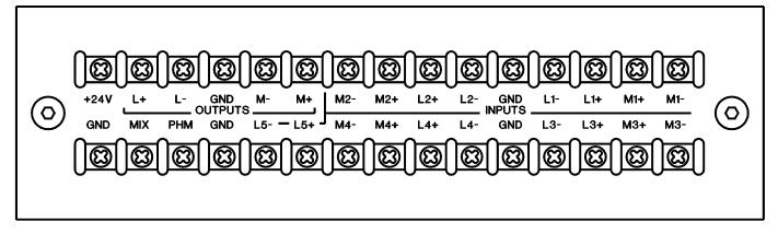
**AUDIO INPUTS:** Inputs are labeled **1** through **5**., **L** is for line level inputs, **M** is for mic level inputs. You may use either the mic or line terminals for inputs 1-4, Input 5 is line only. Both may not be used simultaneously. Connect balanced audio to **+**, **-**, and ground. Connect unbalanced audio to **+** terminal; connect **-** to ground terminal together with the unbalanced shield.
