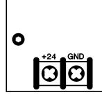
**POWER CONNECTION**: Connect a single-ended 24vdc power source to the +24Vdc terminal. Connect the ground return from that supply to the adjacent ground terminal. Power supply and circuit grounds are common.
