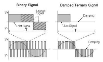
In tests using the same hardware configured for ternary and then for binary, ternary's high frequency energy at zero output is attenuated over 20 dB below binary operating into the same filter! This means higher efficiency and smaller filter components.
