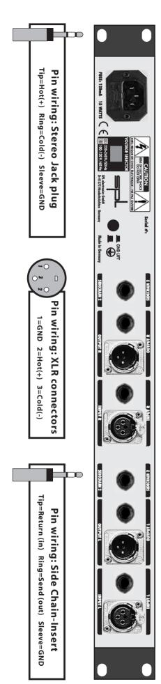
DYNAMAXX is fitted with both XLR-connectors and TRS stereo jacks for balanced operation, though the jacks may be used with unbalanced connections simply by plugging in mono jack-plugs. The level difference that normally occurs when a balanced input or output is used unbalanced is automatically compensated for.
