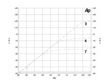
The EFFECT-COMPRESSION function applies a fixed Release time of 60ms, but the Attack time is still automated. This mode increases the perceived loudness in comparison with the normal Compression mode, and audible compression artifacts can be generated for creative purposes.
