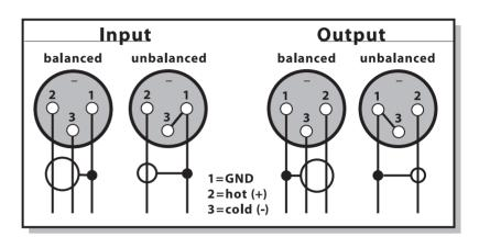
Both output stages operate in parallel, so it is possible to connect two different destination units simultaneously, for example to record to two different media at the same time or split the output between a mixer and effects processor. However, only one type of input (jack or XLR) should be connected at a time – the DynaMaxx is not intended to be used as a mixer!
