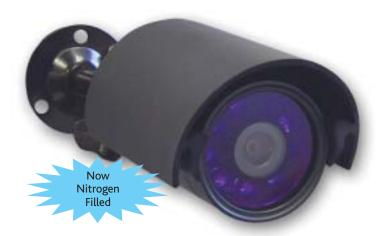
Our B/W waterproof CCTV camera is 100% waterproof with underwater operation capabilities to 90 feet. It features a 3.6mm fixed focus lens, CDS sensors 10 infrared LEDS, and built-in electronic iris. It is encased in a brass housing that is painted black and comes with a clip-on sunshield. A mounting bracket, 120 ft cable and a 12V DC power supply are included. This model is nitrogen filled to eliminate condensation.
