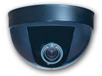
This 1/3" B/W varifocal dome camera features an adjustable 4-9mm lens with a built-in electronic shutter. The camera can rotate 360 degrees. It has 0.02 lux low light sensitivity with 420 lines of resolution. A 12V DC power supply is included. A color version of this camera can be found under model number CVC-6405DC.
