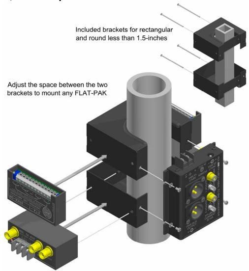
The PM-1V is designed to mount any RDL FLAT-PAK module to a projector pole. This is a vertical mounting system designed to grip a standard 1-1/2" I.D. pole common to most projector mounts. An included pair of bracket and screw sets allows mounting to poles smaller than 1-1/2" and to square or rectangular projector mounts. Adequate vertical pole clearance must be available for mounting the PM-1V. The bracket side plates are intended for the mounting of any RDL STICK-ON or TX series module.
