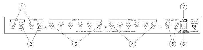
1. LEFT & RIGHT MASTER INPUTS. These are balanced Tip-Ring-Sleeve (TRS) 1/4" Inputs. These Inputs feed all six MONO OUTs when all MONO INs are not used. Connecting to individual MONO INs disconnects that channel from these Inputs (refer to the Block Diagram found on the SM 26B Data Sheet). For unbalanced operation use a standard mono 1/4" plug; for balanced operation use a TRS (stereo) 1/4" plug wired as follows:
