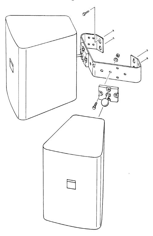
**Important:** Place washer over the screw in back of the bracket, then place the lock nut over the screw and tighten.
