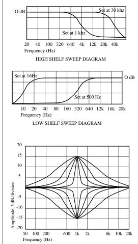
The two shelving filters are designed to tailor the frequency response of the signal; the Low Shelf cuts the frequencies 3 dB at the control's indicated setting and rolls off below, and the High Shelf cuts the frequencies 3dB at the indicated setting and rolls off above.
