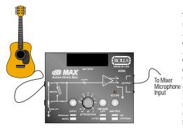
This example shows the ADi6 connected to an instrument. The INPUT switch is *in*, the unused 1/4" jack may be connected to an instrument tuner. The ATTENUATION is at 0 dB, and the GROUND LIFT is *in* meaning the chassis ground is connected to pin 1 of the XLR jack. If the unit is to be powered via 9 volt battery, the BATTERY switch should be *in*, if the unit is powered via phantom power from the mixer, the BATTERY switch should be *out*.
