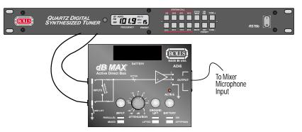
This example shows the mixing capabilities of the ADi6. A stereo source is shown connected to both 1/4" inputs, and the INPUT switch is out. This mixes the right and left signals to mono, and balances the combined signal to be sent to a mixer. The ATTENUATION control, GROUND LIFT switch, and BATTERY switch should all be set for proper operation.
