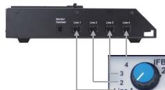
**9.** Use the IFB 1-4 rotary switches to select which phone line audio will be sent to the corresponding IFB XLR output jack.
