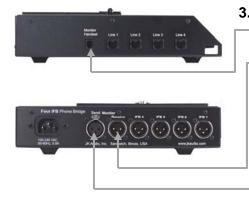
3. Connect a handset to the monitor handset jack and/or connect the Monitor Send and Receive XLR jacks to your audio equipment for communication.
