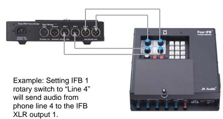
**10.** Adjust audio levels as needed using corresponding volume controls.
