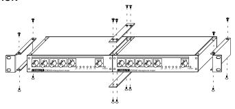
After attaching the brackets, mount the unit in an equipment rack using the supplied rackmount screws and plastic washers.
