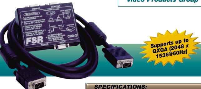
The CDA-2 is a computer video distribution amplifier. It takes the input signal from the video card of a computer and splits it to be used by a projector and a monitor. This unit not only splits the signal it also buffers it to ensure absolute signal integrity at the receiving device (projector or monitor). With 300 MHz of bandwidth, the CDA-2 can support up to a QXGA (2048 x 1536 @ 60Hz) computer video signal approximately 50 feet using high resolution cable.
