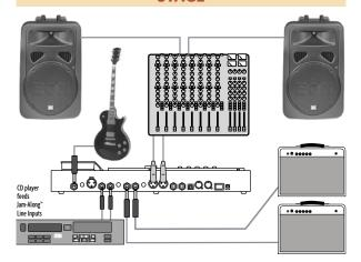
Separate 1/4" & XLR outputs send sound to both the amp and PA
