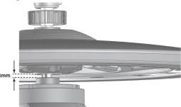
\* Although the gap can be adjusted to a clearance that makes playing the hi-hat easier, setting too narrow or wide a gap can cause improper function of the unit and prevent the hi-hat from sounding as you intend. Setting the gap to 3 mm provides the most natural feel when playing the VH-10.
