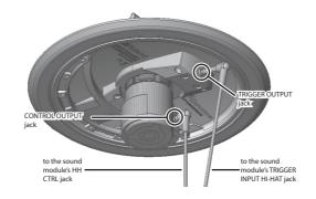
\* Use stereo (TRS) cables to make the connections. If mono cables are used, edge shots cannot be supported.
