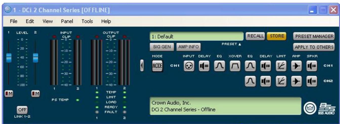
Figure 16 With the "Y 1+2" box checked, both output Ch.1 and Ch.2 are fed by input Ch.1 and input processing is organized accordingly.
