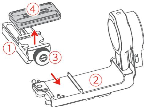
Step 2: Mount camera on ARCA quick release plate **④**.
