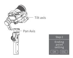
(4) Gimbal rotate automatically from the start position to the end position Gimbal return the start initial position after setting, and then tilt and pan axis will start to rotate according to the parameter that has been set.
