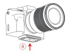
Step 3: Insert ARCA quick release plate directly into quick release plate 1 , tighten the safety lock 3 for ARCA quick release plate.
