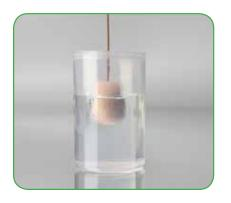
The H7 Headset includes a waterresistant windscreen coated with a superhydrophobic nanocoating to repel water and sweat. This coating is robust but may lose some of its properties after repeated washing. Use only soap and water when cleaning the H7 windscreen.
