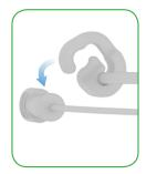
Unclip the boom from the clips along the back of the headset.
