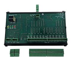
The DMX12ANL-DIN is a 12 channel DMX512 to analog 0-10V interface. It uses pluggable terminal blocks for the DMX512 in and thru connections, analog outputs, and DC power input. The device mounts on standard 35mm "top hat" DIN rail. It is powered by 12 to 24VDC. The DMX12ANL-DIN can be pre-mounted in a NEMA1 electrical enclosure (model DMX12ANL-DIN-JBOX). If a power supply is needed in the enclosure, use model DMX12ANL-DIN-JBOX-PS.
