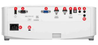
1. USB (service) 5. HDMI 1.4a 2.RS-232C 6. USB Power 3. VGA 7. Audio-In 4. HDMI 2.0 8. Optical S/PDIF
