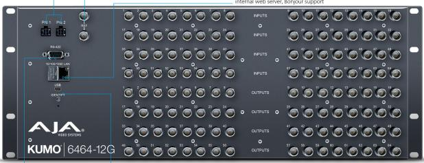
RS-422 RS-422 remote control via 9-pin D-connector with basic support for Grass Valley Native Protocol support USB Connection USB port to easily configure the router IP address and simplify network configurations 12G/6G/3G/HD/SD-SDI Inputs and Outputs All inputs and outputs, 12G/6G/3G/HD/SD-SDI (SMPTE-259/292/424/2081/2082)
