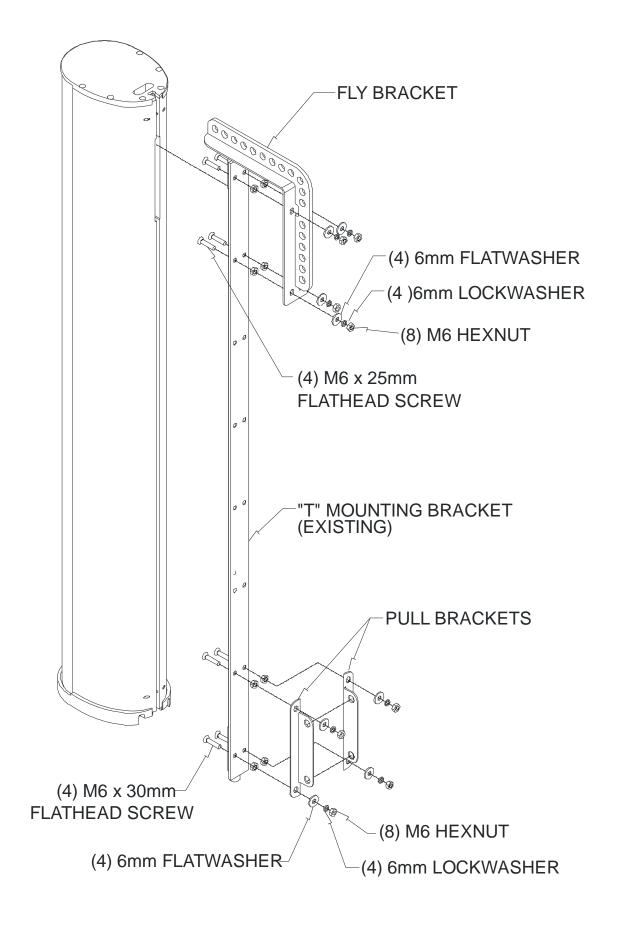
Figure 3: Fly Kit Suspension (Examples)
