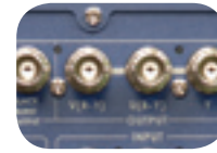
Component Video (Y/R-Y/B-Y) and Black Burst Output
