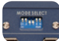
Dip Switches PALB/NTSC, 0/7.5 IRE
