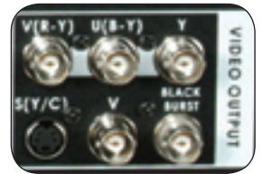
Video Outputs Component, Y/C (S-Video), Composite Video.
