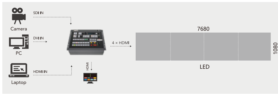
Example: 8K PGM output canvas with all four HDMI PGM outputs spliced.
