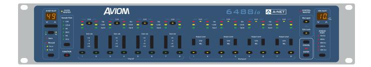
The 6488io provides eight balanced line-level analog inputs to and eight balanced mic- or line-level analog outputs from a Pro64™ A-Net° audio network. The 6488io is ideally suited for low-channel-count network drops, system expansion, and comm links. It is the perfect addition to a small post-production room, radio facility, or snake rack.
