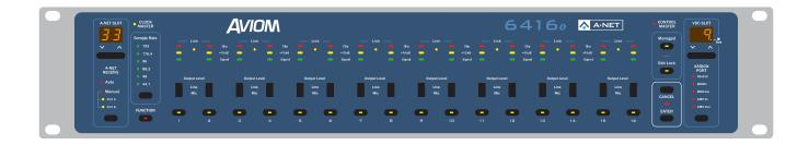
The 64160 Output Module provides 16 balanced mic- or line-level analog outputs from a Pro64<sup>™</sup> A-Net<sup>®</sup> network. Each channel includes a two-position output level switch (mic or line) and three-segment level metering. Alternate analog audio outputs are provided via DB25 multipin connectors on the rear panel.
