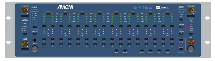
The remote-controllable 6416m Mic Input Module provides 16 balanced miclevel analog inputs to a Pro64™ system. With a switchable pad per channel, the 6416m also accepts balanced line-level inputs. Each channel features continuous gain control, +48V phantom power, low cut filter, phase invert, and a network activation button.
